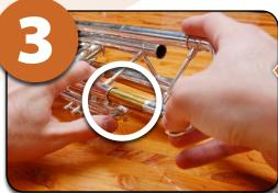
Slide the crook from the lower tuning slide receiver keeping the new leadpipe intact. This should relieve tension on the new leadpipe making it easier to remove it from the **Leadpipe Stabilizer**.
